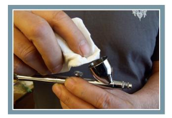
After wiping as clean as possible, squirt airbrush cleaner into the paint reservoir. Spray the cleaner through the airbrush into a rag, paper towel or airbrush spray out pot. Again, wipe the color cup with a paper towel. Use a dental brush to reach into the nooks and crannies of the color cup with the cleaner.
