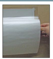
Reach underneath the frisket film and grab the loose sheet of backing paper.
