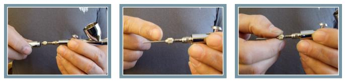
Once the color cup is cleaned, remove the airbrush handle to expose the needle. Notice that there is a nut holding the needle in place. This is called the needle chuck nut and it must be loosened to remove the needle.
