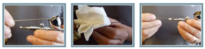
Once the needle is removed, wipe off paint residue with a paper towel. Always wipe the needle from the end to the tip and be careful not to stick yourself, since it is sharp. Once the needle is clean, replace it in the airbrush. Slide it back through the needle chuck screw gently pushing it forward until it stops. Do not push it once it stops. Once the needle is back in place, re-tighten the needle chuck nut.
